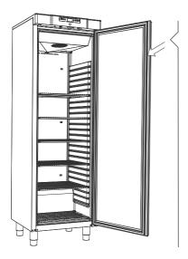
The door gasket should be cleaned regularly with a mild soap solution.
