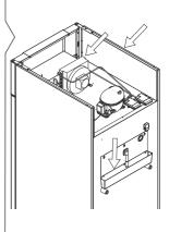
It is recommended that the re-evaporation tray is checked regularly for foreign objects and cleaned accordingly.
