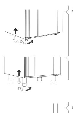
Cabinets equipped with legs should be levelled as shown in the illustrations to the left.
