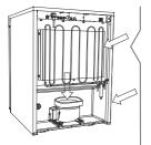
The compressor compartment and in particular the condenser must be kept free from dust and dirt. This is best done with a vacuum cleaner and a brush. Do not flush compressor compartment or evaporator with water as this may cause short circuits in the electrical system.
