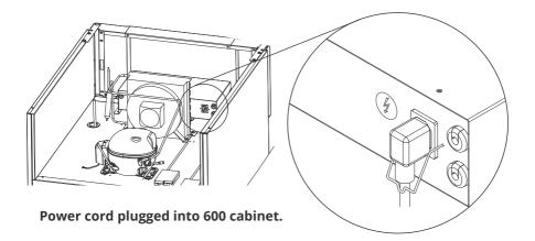
The appliance must be connected to the external power supply using a suitable device which mechanically prevents the plug and socket from being separated unintentionally. The connection must be labelled:
